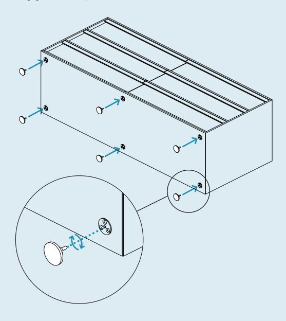
INSTALL ANTI-TIP BRACKETS TO CASE.
